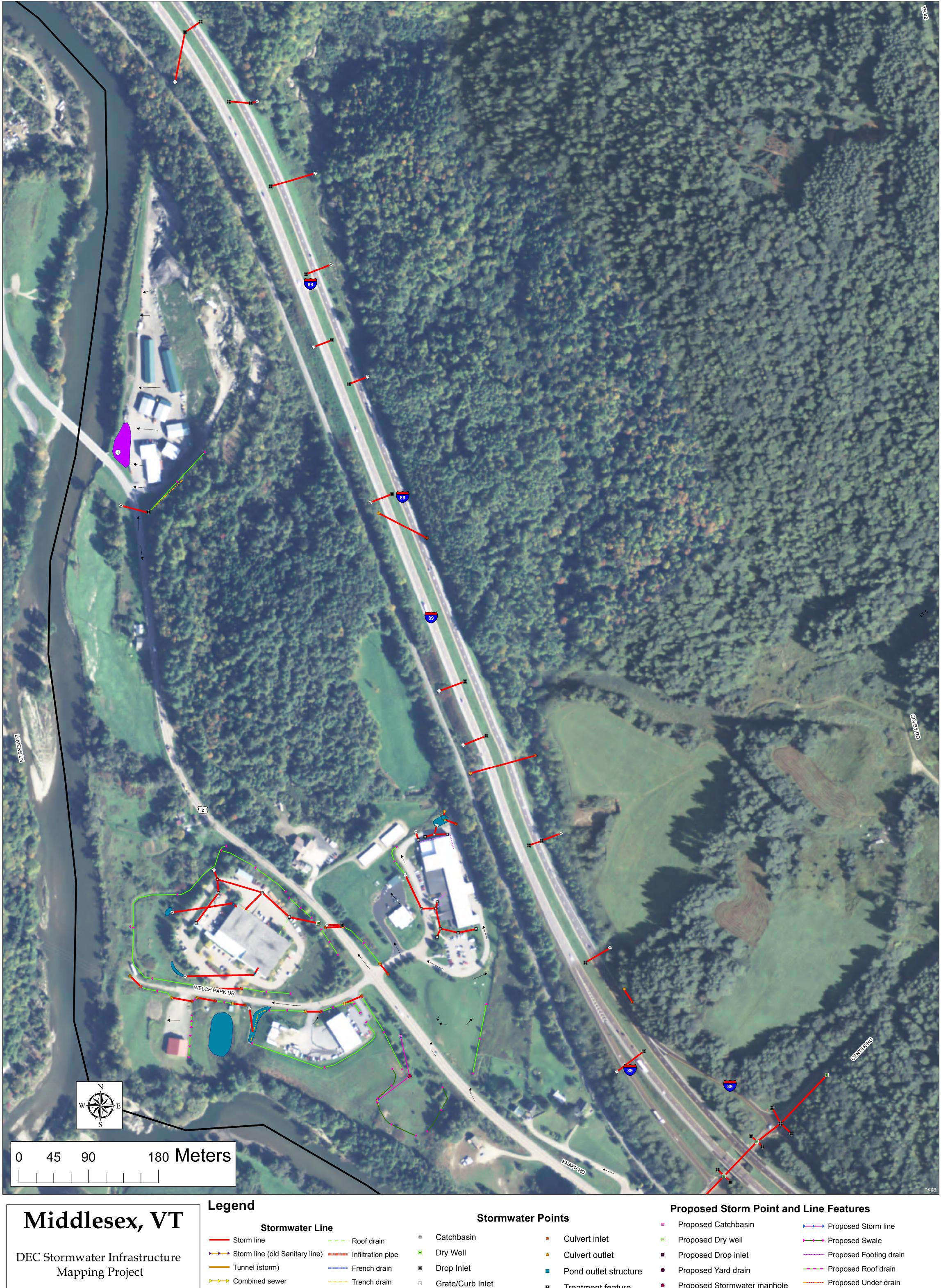
This map shows the connectedness of the stormwater infrastructure and was compiled from various sources including Town plans, WWMD plans, Stormwater permit plans, municipal member knowledge, field data, and a mapping grade GPS.
